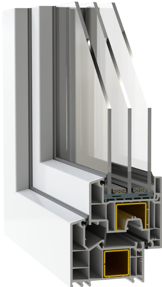
Decco 84MD is a modern system with an installation depth of 81 mm and a third flexible center seal, offering extended reinforcement chambers to increase the windows' rigidity. Thanks to its optimum profile height, the system provides up to 5% more light than other solutions in its class. Moreover, it includes transition profiles for large sliding and balcony doors and allows the use of bonded glass technology, increasing stability and enabling the creation of larger structures.
